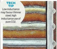
Some welders have variable inductance (the rate at which volts and amps alternate). High 90% inductance (middle) produces a 'wetter' flatter bead; vice versa for low 10% inductance (top). Most welders are set as standard to 35% (bottom).
