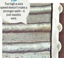
The top bead is too slow; the middle is too fast; and the bottom is as recommended. It's difficult not to compensate by moving the torch at a different speed, so the results are subtle. There's a clear variation in bead height, however.
