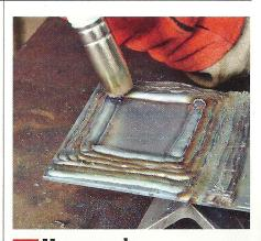
Weld successive beads on a steel plate.
